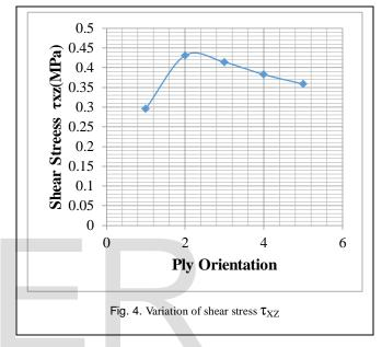
Maximum variation in the values of normal stress and the shear stresses can be seen in between the first and the second orientation i.e. for the orientation [0/0/0/0] and [0/30/30/0] stresses vary considerably.
